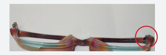
The spring of the broad hinge (Sigma 4,6, FlexUno) can just break by massive force influence.
