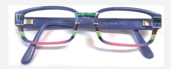
The frame is not broken at color change, but got totally damaged by heat.
